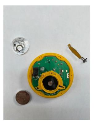
4. <u>Important</u> Discharge any remaining current from the watch. Do this by using the tweezers supplied, place one leg of the tweezer where the battery coil is sited and the other on the battery housing below the battery arm (see photo).
