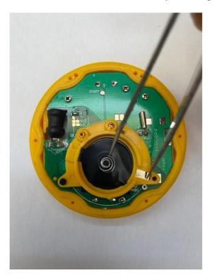
5. Insert the new battery with the positive side / text side facing up. Handle the new battery as little as possible, holding it on the sides. If necessary, wipe with a soft cloth
