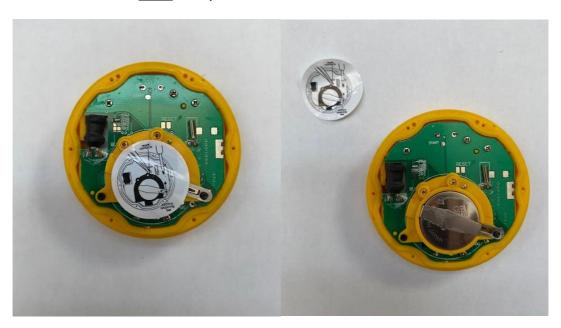
3. Loosen the battery retaining bar and remove the old battery
